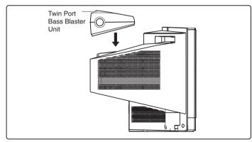
2 Firmly insert the Twin Port Bass Blaster Unit connector into the BASS SPEAKER OUT terminal.
