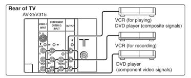
When you use VIDEO-1 INPUT, you should choose to connect S-VIDEO or video input. If S-VIDEO connector and video input are connected at the same time, no picture displays on the screen and the message "PLEASE DISCONNECT VIDEO-1 CABLE!" appears. In this case, you should disconnect either S-VIDEO or video input.
